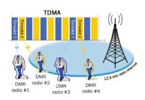
These possibilities give the customer greater flexibility of usage of the resources, sharing the same radio channel for different voice or data services in a completely transparent way for the users.
